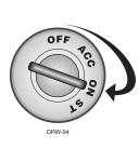
To disarm the security system, turn the ignition to the ON position. Press the Valet button the preset number of times (one to five times) within 15 seconds. After five seconds, the system will disarm. If the system does not disarm, you may have waited too long; turn the ignition off and on and try again.
